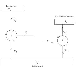
For the composite engine use the usual formula for efficiency, in terms of the **net** work done on the surroundings and the (heat) energy supplied at the **highest** temperature. Then exploit the relationships between heat flows and temperatures.
