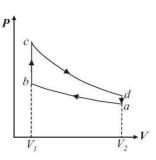
The 'Otto cycle' is an idealisation of the internal combustion engine. Which segments represent fuel compression, burning, and exhaust?
