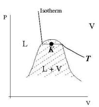
The figure shows an isotherm on the P-V projection. At the point X the substance is a mixture of liquid and vapour. The total mass of substance is the sum of the liquid and vapour masses  $m=m_l+m_v$ . At coexistence  $v_l$  and  $v_v$  are the specific volumes of the liquid and vapour (per kg).
